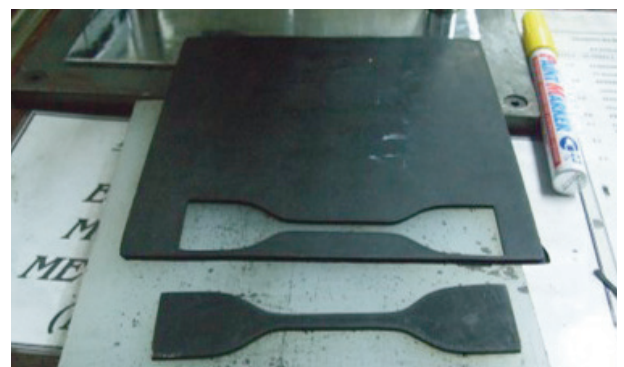
Test sample made from specimen taken from final compound
